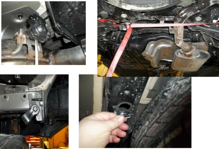
4. Run the M10 bolts into existing weldnuts in frame rail to remove any debris. Remove bolts.
