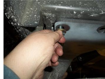
7. Install remaining conical washers and hex nut onto matching bolts.
