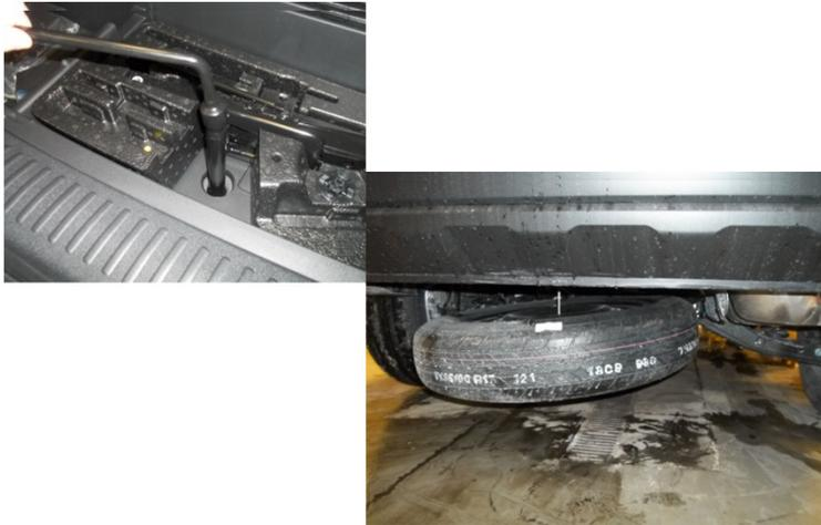
2. Remove the driver side rear plastic cover, located underneath the vehicle, by using a small Phillips head screwdriver to remove fasteners, also remove (5) plastic push pins and (2) nuts.
