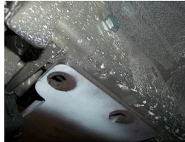
6. Insert M10 bolts (item 8 & 7) through bracket and into the frame as shown in Figure 1 (Hand tighten).
