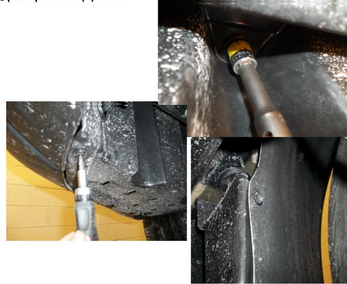
3. Lower exhaust by removing the rear and side hangers, support the exhaust to prevent damage. Spraying a lubricant or soapy water on the metal hanger rod and the rubber isolator helps removal. Remove rubber plugs from bottom of frame rail. Both sides
