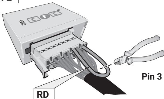
Pin 3 and Pin 2 disconnected
