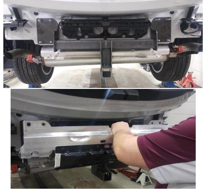
**6. Tighten all fasteners to torque specifications. Tighten all M12 fasteners with torque wrench to 65 Lb.-Ft. (88 N\*M)**
