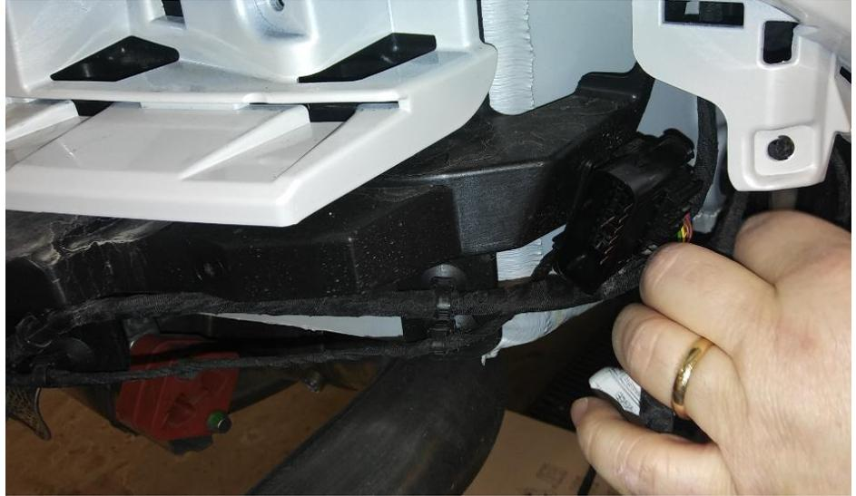
**2. Lower exhaust and disconnect sensor wiring:** Use a 13mm socket to remove 2 nuts from the exhaust (1 each side). Next disconnect the back-up sensor wiring and hands free sensor (Not shown). Lower tailgate to access upper mounting fasteners.
